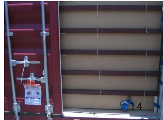
Cable tied top after lockdown for top and bottom, lower bar with warning stickers. To discourage left door opening when container is loaded.
